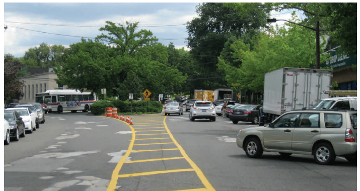
“Before” looking at Welwyn Road and Shoreward Drive with only a painted median between vehicles; a dangerous condition.
